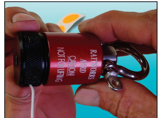
Holding base and body, screw together by turning red body until firmly seated.
