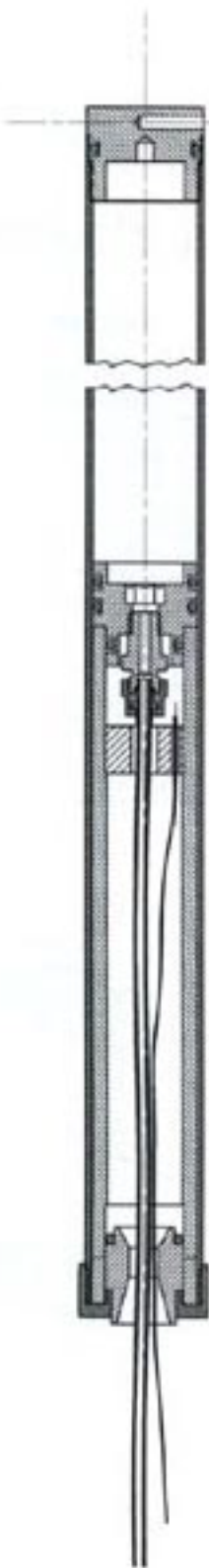
Cut-Away View of Properly Assembled Motor
