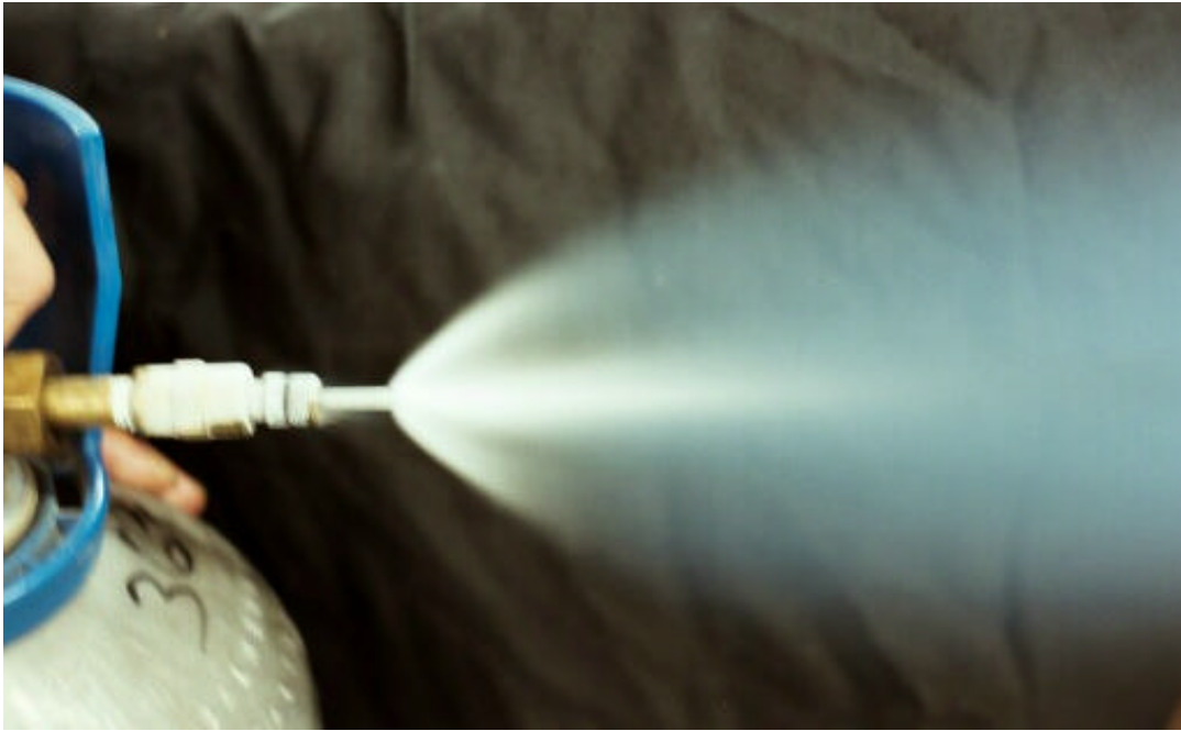
K-240 U-C Valve #3 Star Pattern 6 Slots PolyPro Grain
