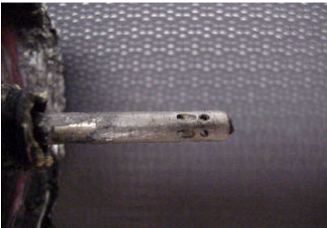
Holy Injector Batman, what happened to the top o-ring and groove? K-240 U-C Valve #5 90 degree injector 12 holes PolyPro Grain
