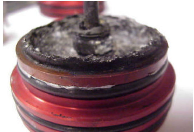
Holy Injector Batman, what happened to the top o-ring and groove? K-240 U-C Valve #5 90 degree injector 12 holes PolyPro Grain
